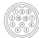
H connector (12 pin) - M23 CCW Hummel 7.410.000000 - 7.002.912.603 solder side view FV
